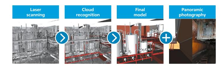
Application of the digital product "Digital Operating Engineering Radiation Model" (DOREM) provides a fundamentally new level for development of initial data corresponding to the actual state of the facility. This leads to an increased accuracy of results whilst reducing project staffing. It is based on the application of digital technologies with addition of laser scanning technology and creation of photo panoramas using a spherical photography method.
